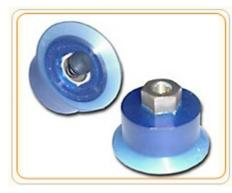
iQ Valves vacuum cup with a built-in check valve was designed for applications where multiple vacuum cups are connected to a main vacuum line but only a portion of the cups are activated at one time. Check valves built into the cups prevent inactivated cups from leaking atmospheric air into the system which would normally reduce the vacuum level in the main line. With these specialty cups, full vacuum is maintained in the main line at all times.
